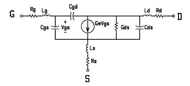
Figure 5.31 Small-signal equivalent circuit of the FET
