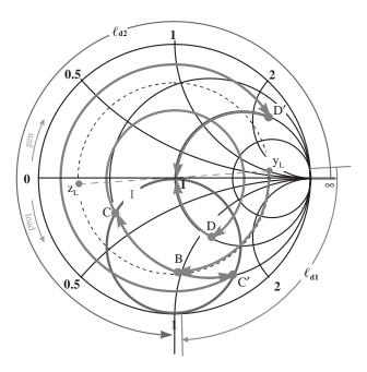
**Figure 3.58** Double stub matching
