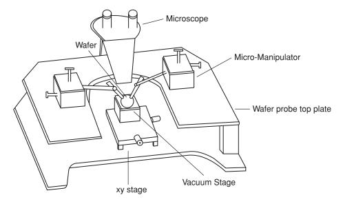
Figure 3.77 Wafer prober with micromanipulators and probes
