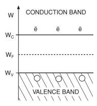
Figure 2.4 Semiconductor energy band diagram
