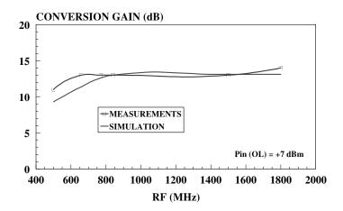
Figure 5.43 Conversion gain vs RF frequency
