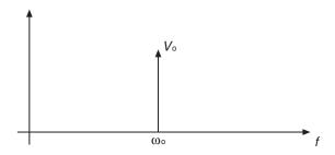
Figure 7.50 Ideal output response of an oscillator
