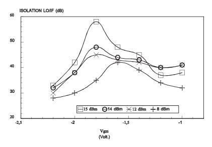
**Figure 5.65** LO/IF isolation vs  $V_{gs}$
