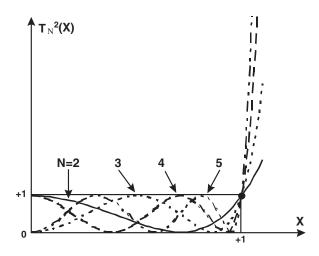
**Figure 6.10** Chebyshev filter response up to N = 5
