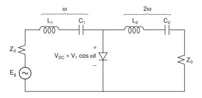
Figure 2.20 Circuit for harmonic generation using varactor diode
