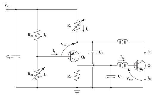
Figure 4.44 Active biasing circuit for bipolar transistors
