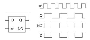
**Figure 7.48** D-flip-flop configured as a divide-by-2
