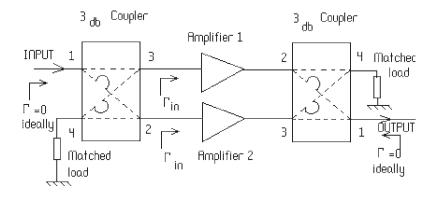
Figure 4.20 Basic balanced amplifier configuration
