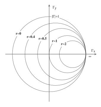
Figure 3.44 Circles of constant normalised resistance, r
