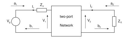
**Figure 3.41** Two-port network terminated at port 2 in  $Z_0$
