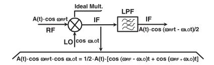
Figure 5.2 Signal components in an ideal mixer
