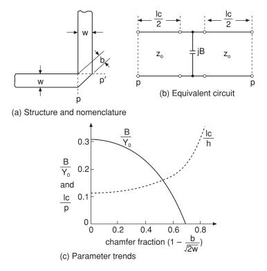
Figure 3.20 The chamfered (or mitred), right-angled, microstrip bend and relationships
