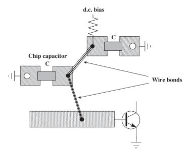
Figure 4.61 Semi-lumped LPF configuration
