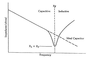
Figure 4.28 Impedance characteristic of a practical capacitor
