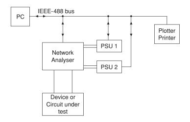
Figure 3.70 Typical equipment configuration for s-parameter measurements
