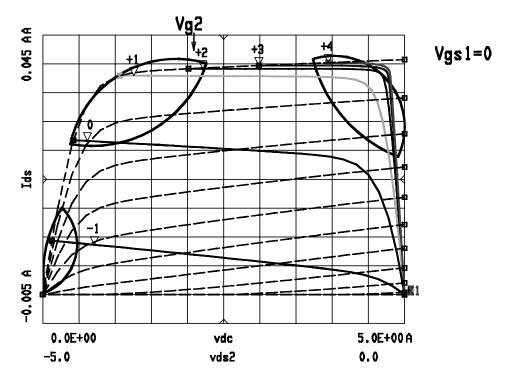
Figure 5.35 I/V Curves of the transistors
