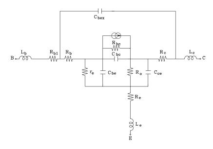
Figure 2.62 Small signal HBT equivalent circuit model
