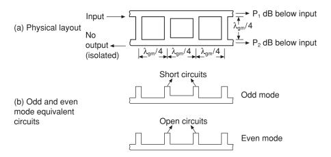
Figure 3.35 The orthogonal branch-line directional coupler
