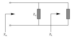
Figure 3.53 Shunt connection of lumped element
