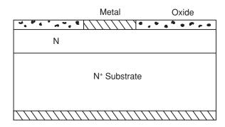
Figure 2.28 Schottky junction structure
