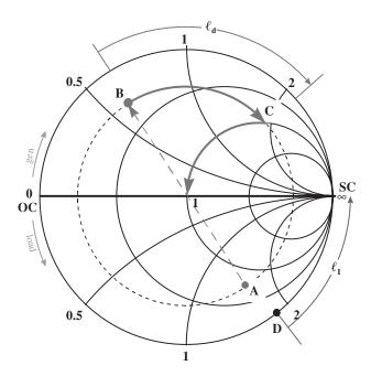
Figure 3.56 Single stub matching
