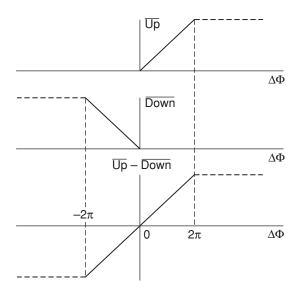
Figure 7.39 Response of digital phase-frequency detector
