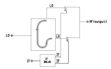
Figure 5.47 Singly balanced HEMT upconverter
