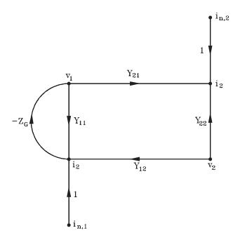
Figure 4.23 Noise model for two-port device
