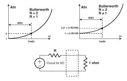
Figure 6.21 Attenuation characteristics of Butterworth PLPF
