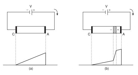
Figure 2.42 Electric potential versus position along Gunn diode: (a) electric field below threshold, (b) electric field above threshold
