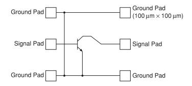
**Figure 3.75** Device layout on a wafer
