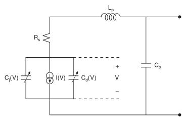
Figure 2.14 Diode equivalent circuit model
