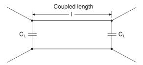
Figure 3.33 Schematic diagram of coupled microstrips, with compensating capacitors across the ends
