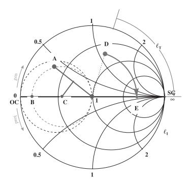
Figure 3.65 Matching using a single section line
