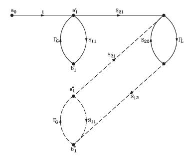
Figure 4.7 Second modified flow graph
