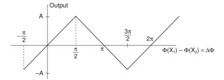
Figure 7.36 Transfer curve of phase detector
