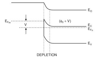
Figure 2.24 Energy band diagram for a Schottky junction
