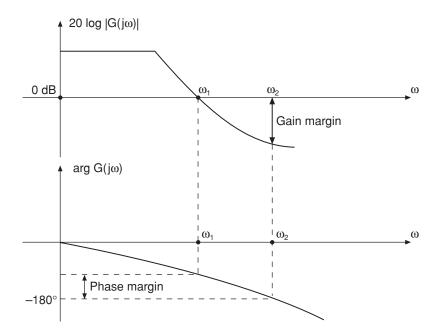
Figure 7.31 Bode plots for an unconditionally stable PLL showing phase and gain margins
