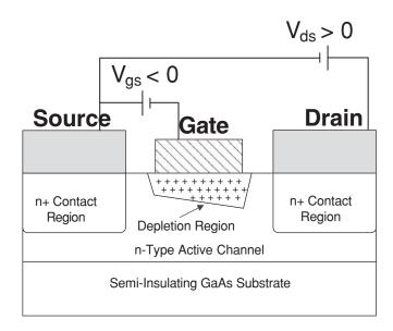
Figure 2.49 GaAs MESFET cross-section
