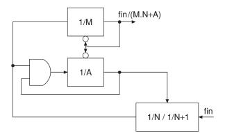
Figure 7.47 Dual modulus divider
