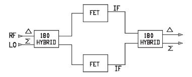
Figure 5.46 180-degree singly balanced FET mixer
