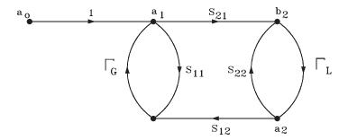
**Figure 4.5** Flow graph for two-port with generator and load
