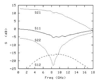
**Figure 4.16** Scattering parameters of the ATF-36163 FET
