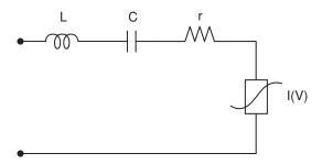
Figure 2.44 Series equivalent circuit model for a Gunn diode incorporating non-linear current source
