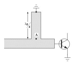
Figure 4.55 Quarter wavelength line configuration
