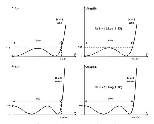
**Figure 6.11** Chebyshev filter attenuation for N = 3 and 4
