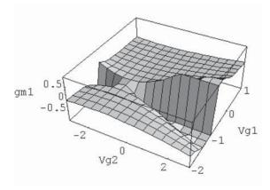
**Figure 5.36** Variation of  $g_{m1}$  (FET1) versus  $V_{g1}$  and  $V_{g2}$
