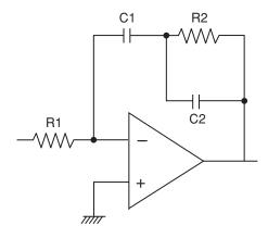
Figure 7.44 Circuit diagram of 2-pole filter
