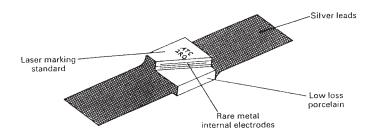
Figure 4.30 Low loss interdigitated capacitor
