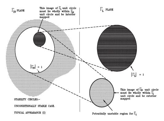
Figure 4.11 Typical appearance of stability circles in the unconditionally stable case
