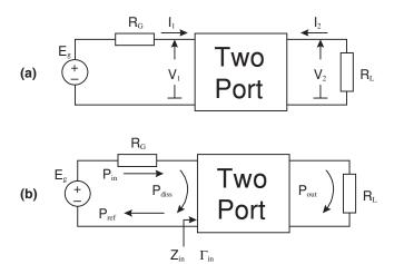
Figure 6.1 Two-port microwave network definitions
