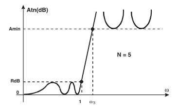
Figure 6.16 Definitions for the Elliptic filter
