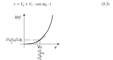
**Figure 5.5** Linearization of the Schottky diode i(v) characteristic
