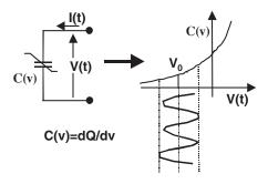
Figure 5.21 Non-linear capacitance under LO excitation
