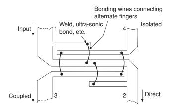
Figure 3.34 The basic form of the Lange coupler
