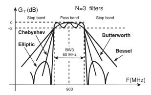
**Figure 6.4** Different filter response types
