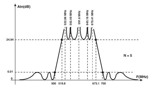
Figure 6.69 Frequency response of Elliptic BS filter
