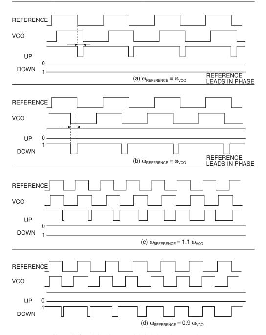
Figure 7.40 Timing diagrams of digital phase-frequency detector
