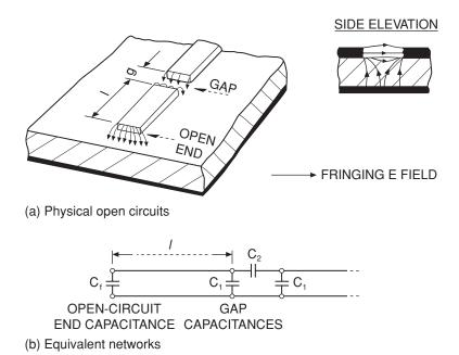
Figure 3.17 Microstrip open end and series gap: (a) physical circuits, (b) equivalent networks
