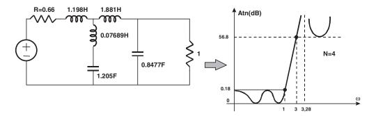
**Figure 6.37** Elliptic filter with N = 4
