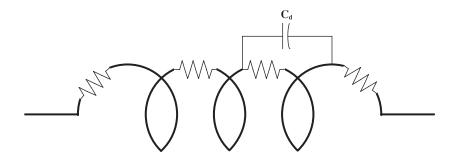
Figure 4.32 Illustration of parasitics on a practical inductor
