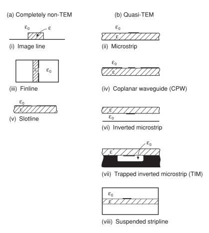
**Figure 3.8** A range of planar and semi-planar transmission line structures suitable as candidates for microwave circuit integration. (Substrates are shown shaded in each case and metal is shown in dense black.)
