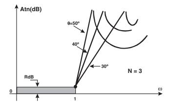
**Figure 6.17** Variation of filter response with  $\theta$
