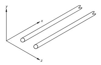
Figure 3.6 Coordinate system for TEM line analysis
