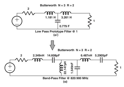
Figure 6.52 Butterworth filter example of LP to BP frequency transformation
