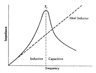
Figure 4.33 Impedance characteristic of inductor
