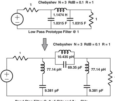
Band Stop Filter @ 0:5 GHz and 7:∞ GHz
