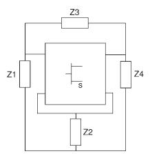
Figure 7.11 Generic topology of a transistor oscillator
