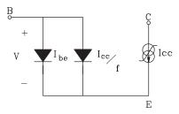
Figure 2.59 DC HBT equivalent circuit under forward bias
