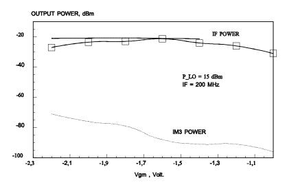
Figure 5.66 Performance of the double-balanced mixer
