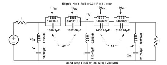
Figure 6.68 Elliptic BS filter including transmission zeros
