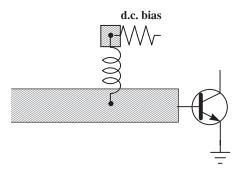
Figure 4.53 Introduction of biasing using practical inductors
