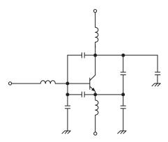
**Figure 3.74** Electrical equivalent circuit of mounting shown in Figure 3.73
