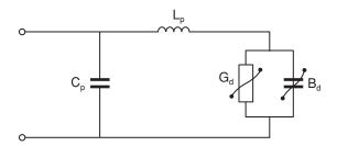
Figure 7.8 Simplified equivalent circuit of a packaged Gunn diode
