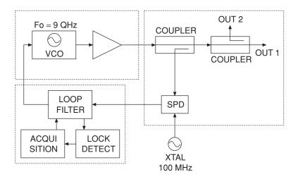
Figure 7.49 9 GHz phase-locked oscillator
