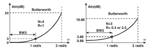
Figure 6.27 Attenuations for Butterworth filters with N = 3 and 4
