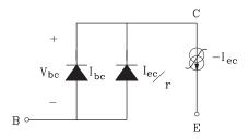
Figure 2.60 DC HBT equivalent circuit under reverse bias
