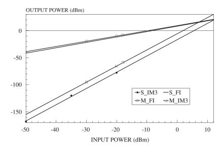
Figure 5.44 Measured and simulated IP3
