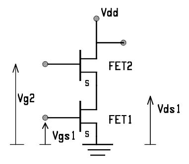
Figure 5.34 Cascade connection for two transistors
