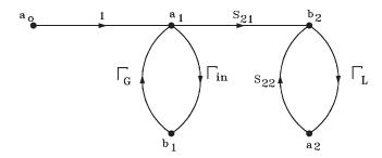
**Figure 4.6** Modified flow graph
