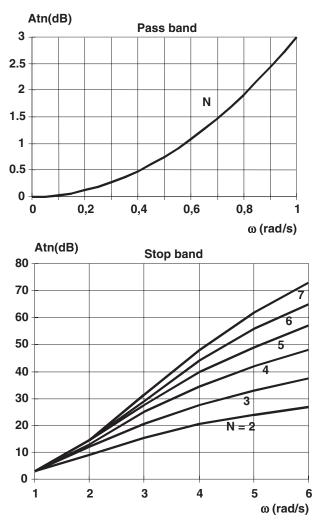
**Figure 6.14** Bessel LPF response for *N* up to 7
