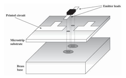
Figure 4.66 Metallic stud through holes
