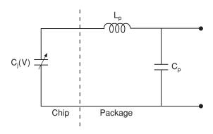
Figure 2.16 Equivalent circuit model of a varactor diode
