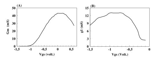
**Figure 5.59** (a)  $g_m$  vs  $V_{gs}$ . (b)  $g_1$  vs  $V_{gs}$
