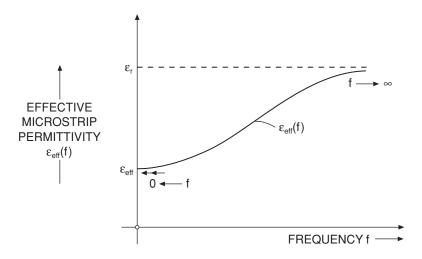
**Figure 3.13** Microstrip dispersion:  $\varepsilon_{eff}(f)$  versus frequency f
