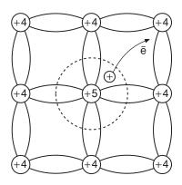
Figure 2.2 N-doped semiconductor crystal
