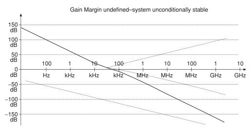
Figure 7.57 Open loop gain with a bandwidth of 50 kHz
