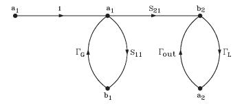
Figure 4.8 Final modification to flow graph
