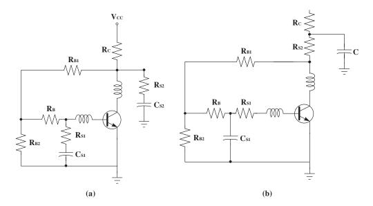
**Figure 4.62** Configuration of stability resistors
