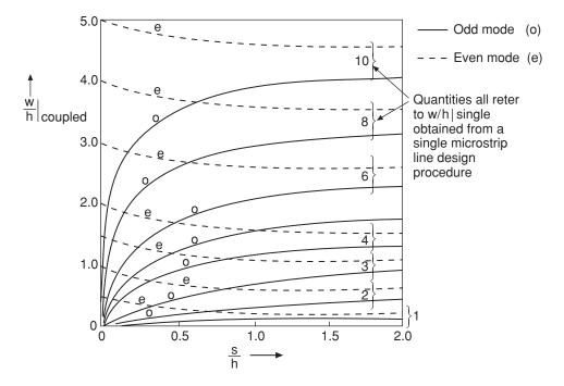
**Figure 3.31** Family of curves for use in the approximate synthesis design (strictly applicable only for  $\varepsilon_r = 6$ )
