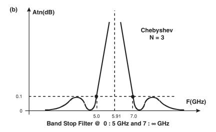
Figure 6.57 Chebyshev LP to BS filter example, impedance transformation
