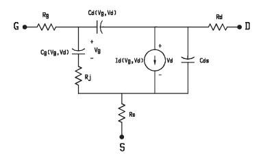
Figure 5.29 Large-signal non-linear MESFET equivalent circuit
