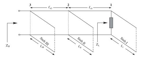
Figure 3.60 Triple stub matching network
