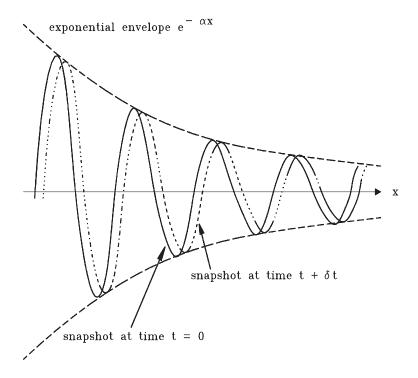
**Figure 3.3** Snapshots of a travelling wave with attenuation
