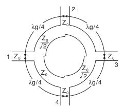
Figure 3.36 The 3 dB ring-form branch-line directional coupler
