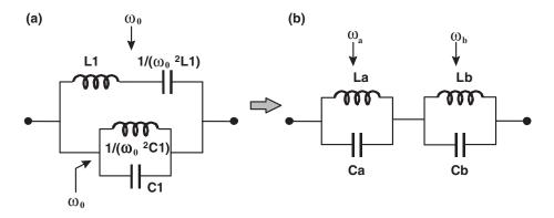
Figure 6.58 Band pass to band stop filter transformation
