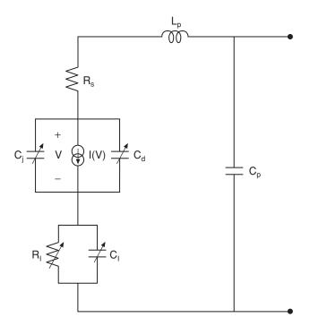
Figure 2.31 Equivalent circuit model for PIN diode
