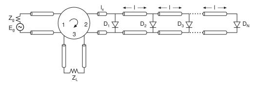
Figure 2.36 High power phase shifter implemented using transmission line, circulator and PIN diodes
