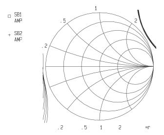
Figure 4.38 Input and output stability circles of the low noise amplifier in the operational bandwidth
