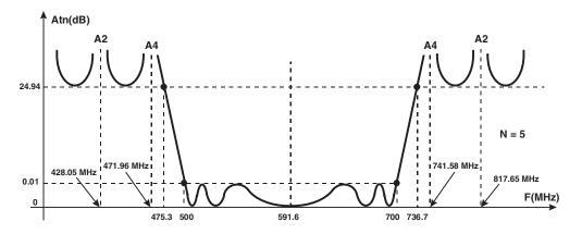
Figure 6.66 Frequency response of Elliptic BP filter
