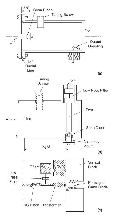
Figure 7.9 Gunn diode oscillators: (a) coaxial mount; (b) waveguide cavity; (c) microstrip
