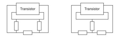
**Figure 7.19**  $\pi$  and T topologies using transmission lines
