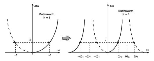
Figure 6.55 Butterworth LP to BS filter example, frequency transformation
