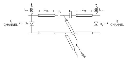
Figure 2.34 Double throw switch implemented by transmission lines and PIN diodes
