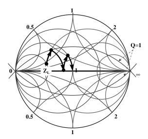
Figure 3.63 Broadband matching using lumped components
