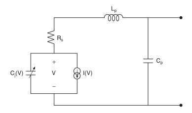
Figure 2.27 Equivalent circuit model for Schottky junction
