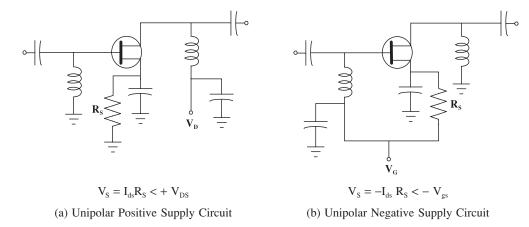
Figure 4.48 Unipolar power supply biasing circuits
