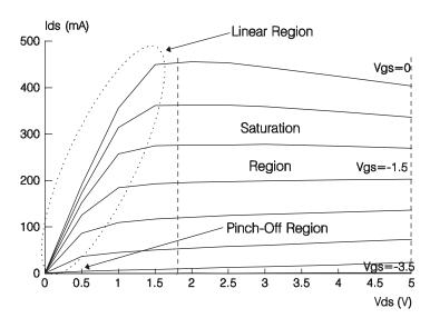
Figure 2.51 Typical I/V curves for a  $10 \times 140 \mu m$  GaAs MESFET device
