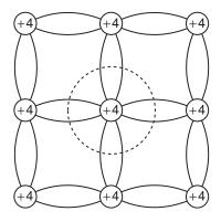
Figure 2.1 Covalent bonding in semiconductor crystal
