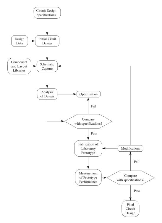
Figure 4.68 CAD RF circuit design procedure
