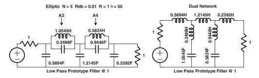
Figure 6.60 Elliptic filter transformation example
