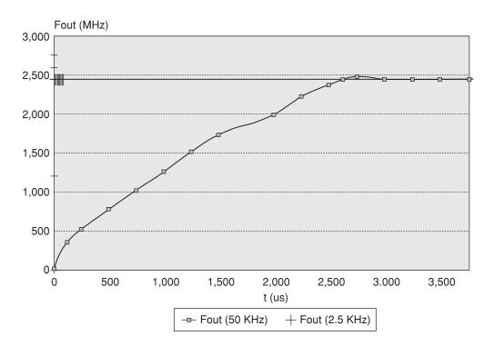
Figure 7.59 Transient responses of two loop configurations
