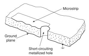
**Figure 3.19** A shunt metallised hole in microstrip (at an otherwise 'open' end)
