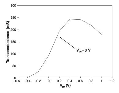
**Figure 2.56** Typical  $g_m$  versus  $v_{gs}$  curves for a  $6 \times 150 \, \mu m$  HEMT
