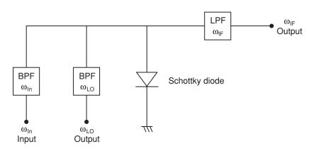
Figure 2.29 Schottky diode used in a mixer implementation
