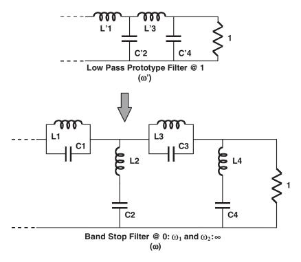
Figure 6.54 Low pass to band stop tranformation
