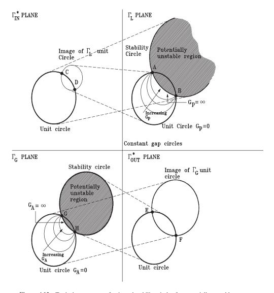
Figure 4.12 Typical appearance of gain and stability circles for potentially unstable two-port
