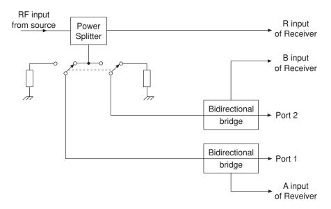
Figure 3.68 Simplified schematic of a two-port test set
