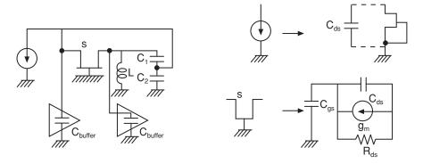
Figure 7.16 Schematic of the Colpitts oscillator used in the calculations
