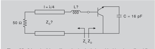
Figure Q3 Schematic of the oscillator, showing the device and load impedances  $Z_D$  and  $Z_L$
