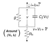
Figure 5.9 Linear equivalent circuit of Schottky diode
