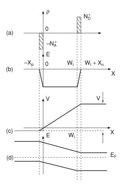
**Figure 2.30** PIN diode charge density distribution (a), electric field distribution (b), potential distribution (c), and energy band diagram (d)
