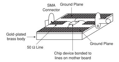
Figure 3.73 Probing a chip device
