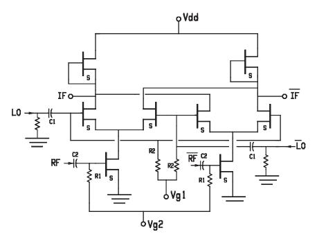
Figure 5.51 Electrical scheme of the mixer
