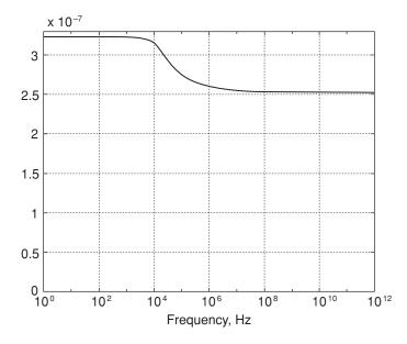
Figure 3.5 Typical variation of line inductance with frequency
