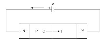
Figure 2.46 Schematic structure of IMPATT diode
