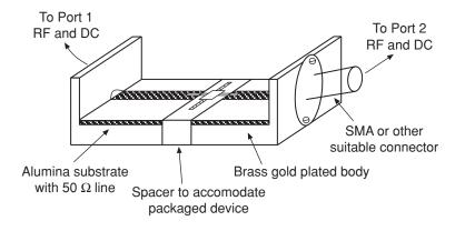
Figure 3.71 Microwave jig for packaged device measurement
