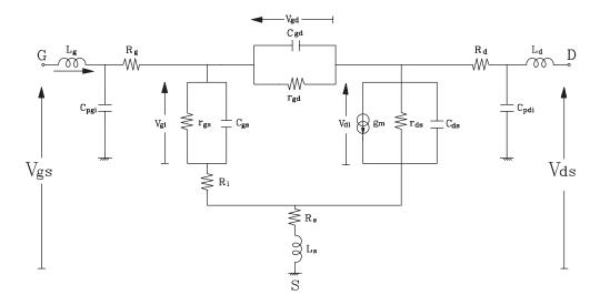
Figure 2.53 Small signal equivalent circuit for GaAs MESFET
