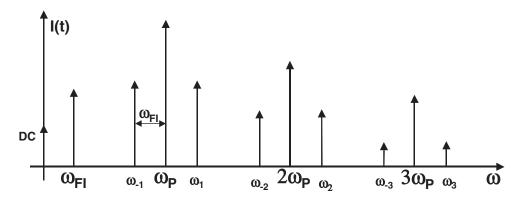
**Figure 5.18** Harmonic representation of the i(t) nonlinear current
