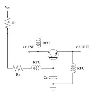
Figure 4.51 Common base configuration
