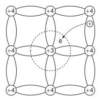
Figure 2.3 P-doped semiconductor crystal
