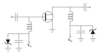
Figure 4.49 GaAs biasing circuit with Zener diodes
