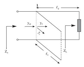
Figure 3.55 Single stub matching network
