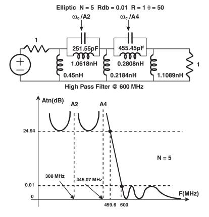
Figure 6.63 Elliptic LP to HP filter transformation
