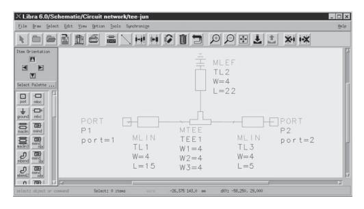
Figure 4.70 Schematic caption of single stub matching network
