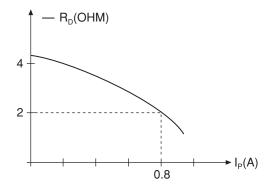
Figure 7.4 IMPATT negative resistance versus RF current
