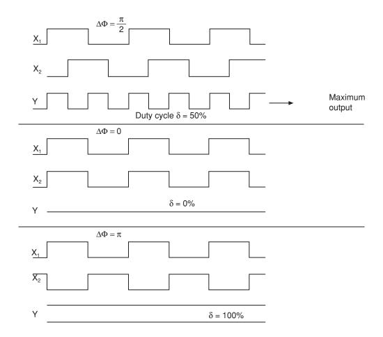
Figure 7.37 Timing diagram of phase detector
