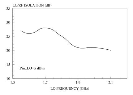
Figure 5.45 LO/RF isolation vs LO frequency
