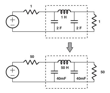
Figure 6.41 Impedance transformation for Butterworth filter
