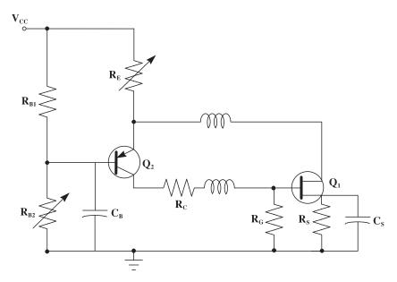
Figure 4.50 Active biasing circuit for GaAs transistors
