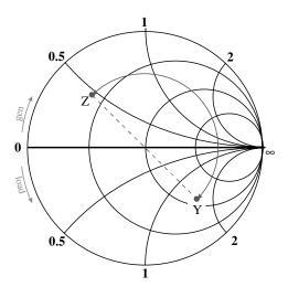
Figure 3.48 Impedance – admittance transformation
