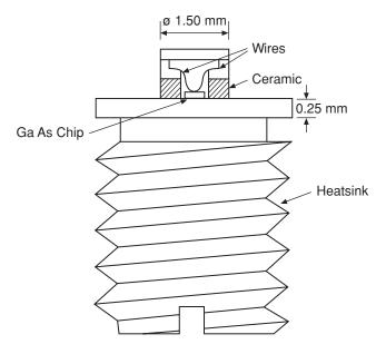
Figure 7.7 Typical packaged Gunn diode
