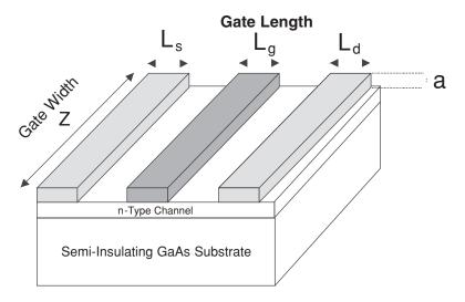
Figure 2.50 Longitudinal view of a GaAs MESFET
