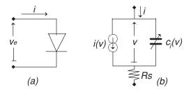
**Figure 5.3** Schottky-Barrier diode equivalent circuit
