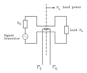
Figure 4.2 Generator connected to a load
