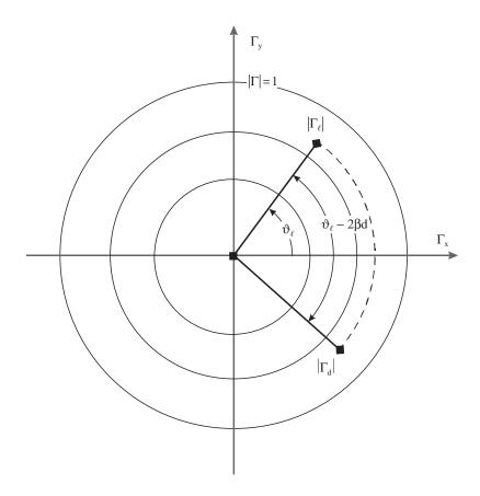
**Figure 3.43** Circles of constant reflection coefficient,  $|\Gamma|$
