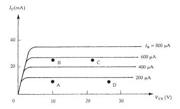
Figure 4.42 Quiescent points for bipolar transistors
