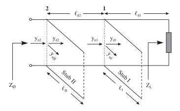
Figure 3.57 Double stub matching network
