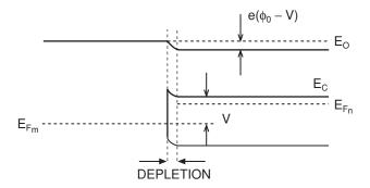
Figure 2.26 Energy band diagram for forward-biased Schottky junction
