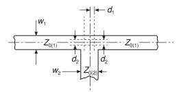
Figure 3.22 Reference planes and impedances for the T-junction
