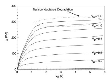
Figure 2.55 Typical I/V curves of a  $6 \times 150 \mu m$  HEMT device
