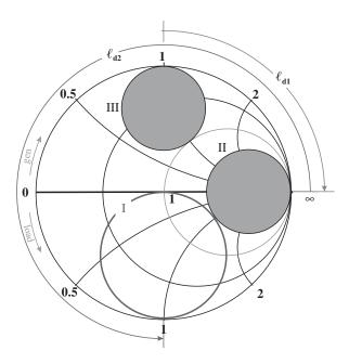
Figure 3.59 Load admittancies that cannot be matched using double stub
