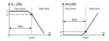
Figure 6.5 Normalised LPF characteristics
