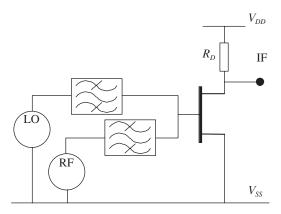
Figure 5.28 FET mixer with RF and LO both applied at the gate
