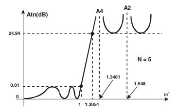
Figure 6.61 Response of filter shown in Figure 6.60
