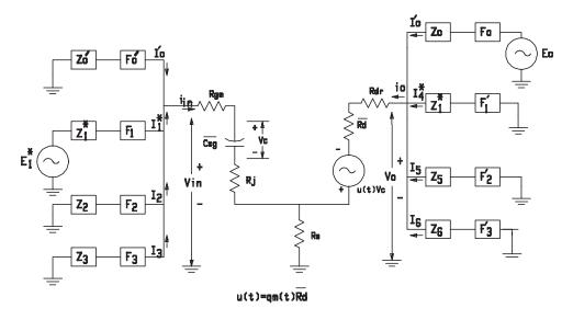
Figure 5.33 Small-signal equivalent circuit of a drain mixer
