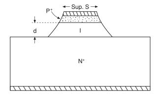
Figure 2.32 PIN diode structure
