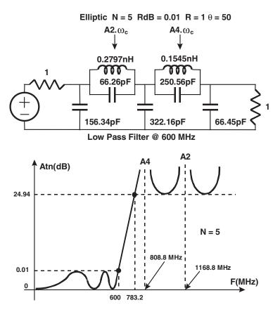
Figure 6.62 Elliptic LP filter transformation
