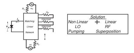
Figure 5.19 Single-diode mixer solution
