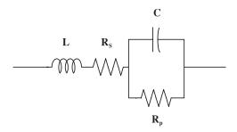
Figure 4.27 Capacitor equivalent circuit
