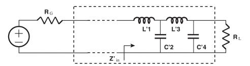
Figure 6.39 Filter network with arbitrary load resistance
