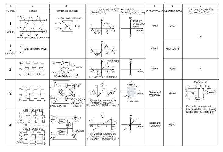
Figure 7.41 Transfer characteristics of four phase detectors
