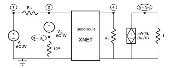
Figure 6.6 PSPICE configuration for generating s-parameters
