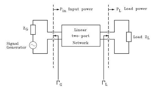
Figure 4.1 Layout of two-port with generator and load
