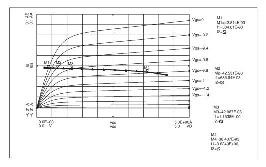
Figure 5.50 I/V DC curves and load line for the T2 transisor
