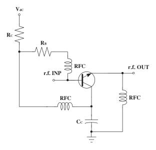
Figure 4.52 Common collector configuration
