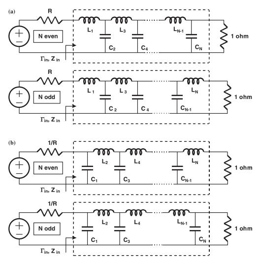
Figure 6.18 Prototype low pass filter definitions
