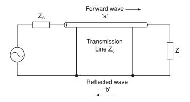
Figure 3.39 Transmission line as a network
