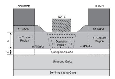
Figure 2.54 Cross-section of a HEMT device
