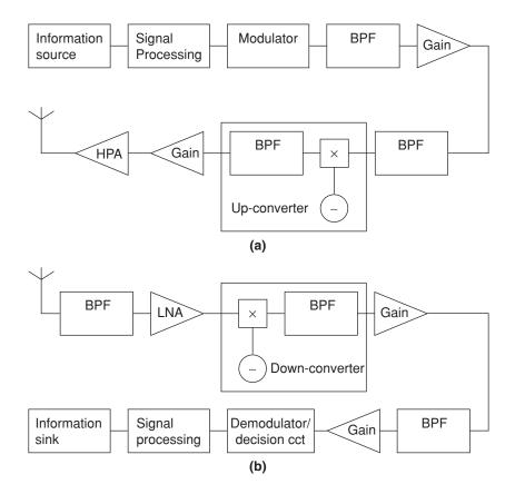
Figure 1.1 Typical microwave communications transmitter (a) and receiver (b)
