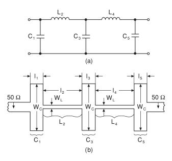
Figure 3.23 Lumped network topology (a) and microstrip configuration (b) for a low-pass filter
