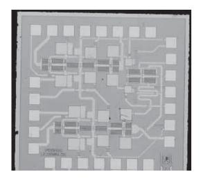
Figure 5.67 The double-balanced mixer
