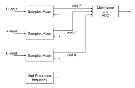
Figure 3.69 Receiver configuration
