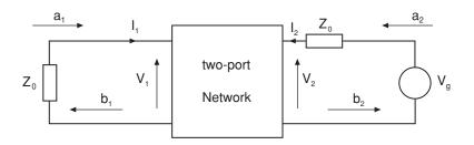
**Figure 3.42** Two-port network terminated at port 1 in  $Z_0$
