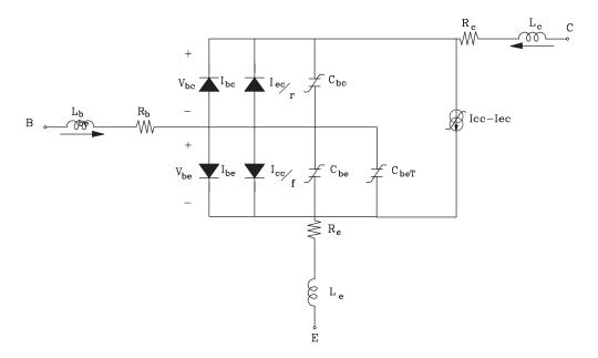
Figure 2.58 Large signal equivalent circuit for HBT
