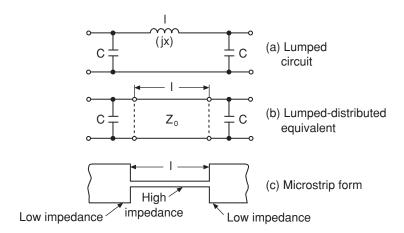
Figure 3.25 Inductive line with adjacent capacitive lines
