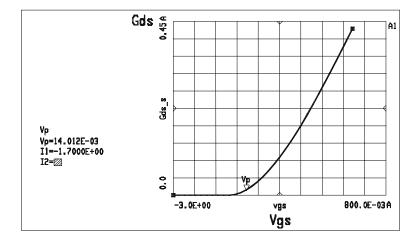
**Figure 5.64**  $G_{ds}$  versus  $V_{gs}$
