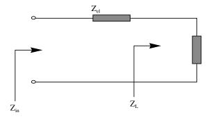
Figure 3.51 Series connection of a lumped element
