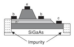
Figure 2.57 Cross-section of a AlGaAs/GaAs device
