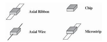
Figure 4.29 Radio frequency capacitor types
