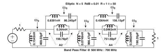
Figure 6.64 Elliptic LP to BP filter transformation
