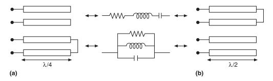
**Figure 7.13** Resonators using transmission lines: (a)  $\lambda/4$  resonators; (b)  $\lambda/2$  resonator
