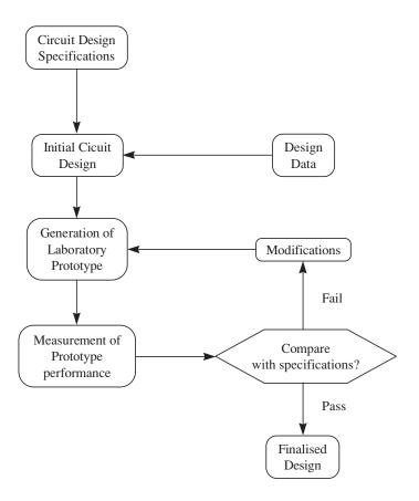
Figure 4.67 Classical RF circuit design approach
