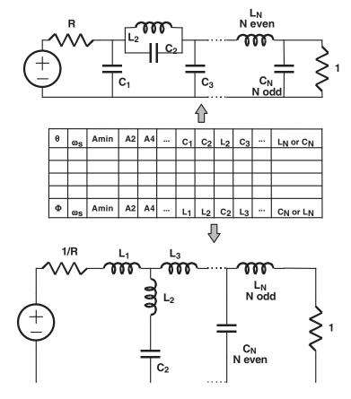
Figure 6.35 Convention for Elliptic filter tables
