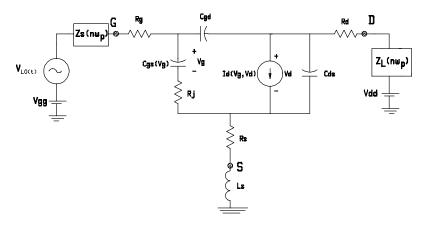
Figure 5.30 Large-signal equivalent circuit of the FET mixer
