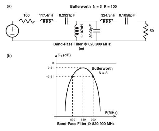
Figure 6.53 Butterworth filter example LP to BP impedance transformation
