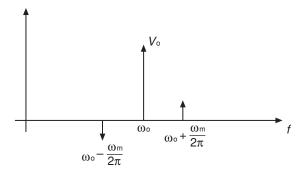
Figure 7.52 Oscillator with sinusoidal modulation
