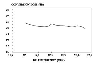
Figure 5.53 Conversion loss of the harmonic mixer
