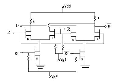
Figure 5.48 Basic structure of a Gilbert cell
