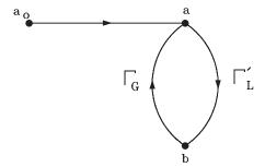
Figure 4.3 Flow graph for generator connected to load
