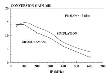
Figure 5.42 Conversion gain vs IF frequency
