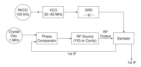
Figure 3.67 Simplified schematic of a signal source
