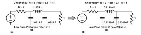
Figure 6.44 Chebyshev filter frequency translation example
