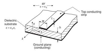
**Figure 3.9** Three-dimensional view of microstrip geometry
