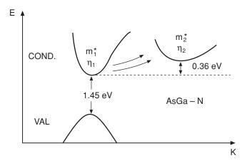
Figure 2.39 Energy band diagram for GaAS
