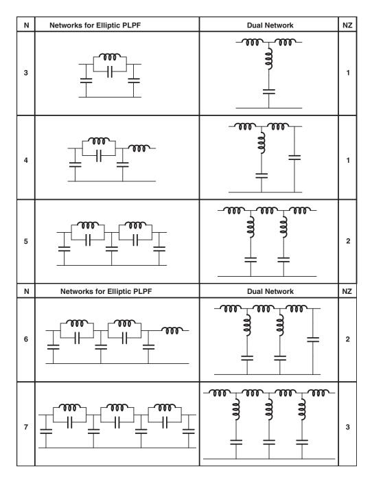
**Figure 6.34** Elliptic networks for N = 3 to 7
