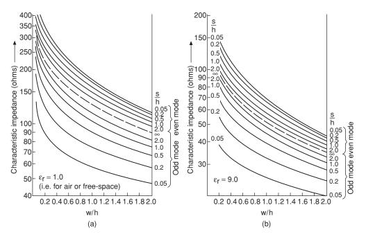
**Figure 3.30** Families of curves for even- and odd-mode characteristic impedances for coupled microstrips in (a) air and (b) on a substrate having relative permittivity 9.0
