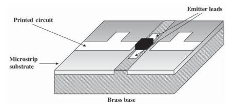
Figure 4.65 Raised ground plane
