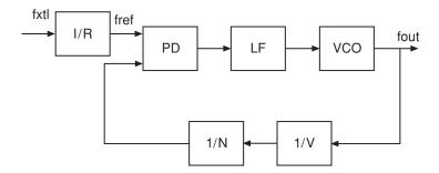
Figure 7.32 Block diagram of phase locked oscillator
