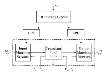
Figure 4.37 Block diagram of amplifier at radio frequencies
