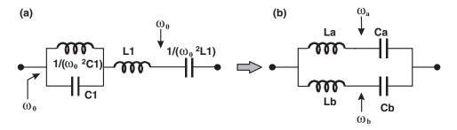
Figure 6.59 Band stop to band pass filter transformation
