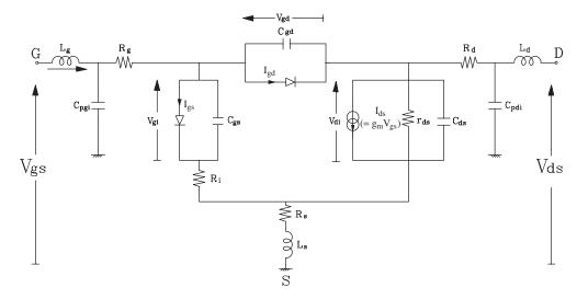
Figure 2.52 Equivalent circuit model for GaAs MESFET
