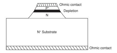
Figure 2.15 Schematic diagram of P-N junction structure
