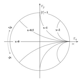
**Figure 3.45** Circles of constant normalised reactance, *x*
