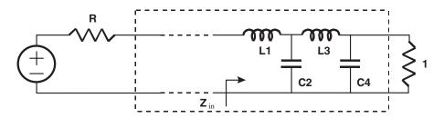
Figure 6.38 Prototype filter ladder network
