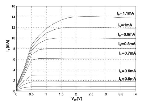
Figure 2.61 Typical I/V curve of a HBT device Note: DEVICE: H67 HBT from Daimler-Benz  $I_b = 0.1$  mA to 1.1 mA, increment 0.1 mA
