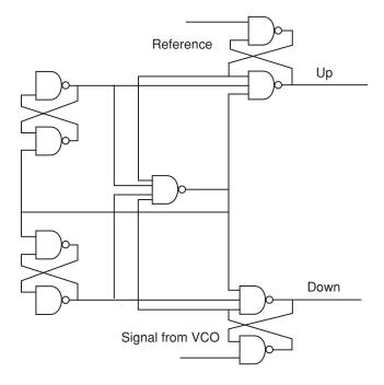
Figure 7.38 Digital phase-frequency detector
