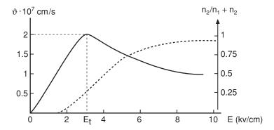
Figure 2.41 Mean electron velocity versus applied electric field
