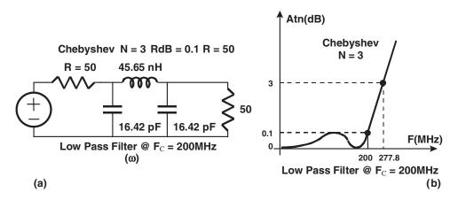
Figure 6.45 LPF frequency and impedance transformation
