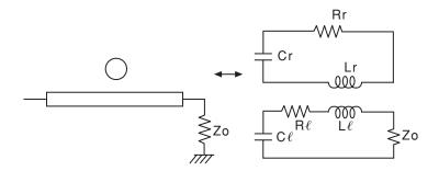
Figure 7.14 Schematic of resonator coupled to a microstrip line
