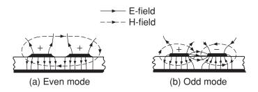
Figure 3.28 Even- and odd-mode field distributions for parallel-coupled microstrips
