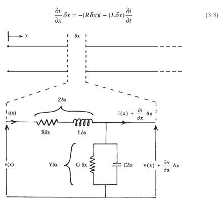
Figure 3.2 Lumped parameter model of an elemental length of transmission line
