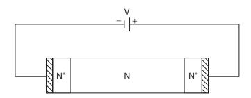
Figure 2.40 Three-layer structure of Gunn diode
