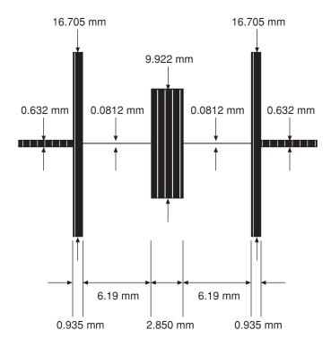
Figure 3.26 Layout of the 2 GHz Butterworth microstrip LPF
