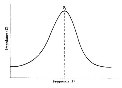
Figure 4.25 Frequency characteristic of a practical resistor
