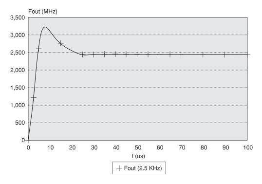
Figure 7.60 Transient response using 2.5 kHz loop showing more detail
