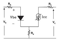
Figure 5.13 One diode simplified circuit under forward bias conditions
