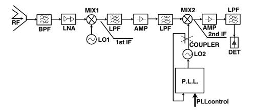
Figure 5.1 Double-mix synthesized receiver
