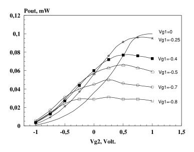
**Figure 5.39** IF output power vs  $V_{e2}$
