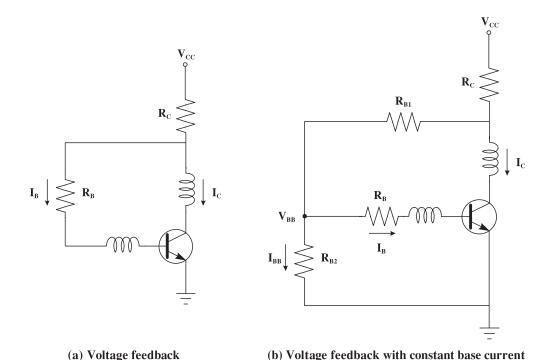
Figure 4.43 Passive biasing circuits for bipolar transistors
