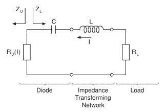
Figure 7.5 Series resonance type IMPATT oscillator circuit
