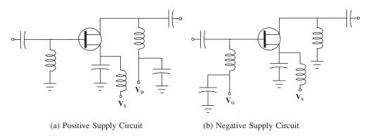
Figure 4.47 Single power supply biasing circuits
