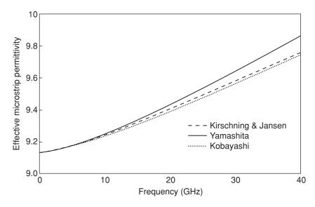
Figure 3.14 Dispersion curves for a microstrip on a GaAs substrate (comparison of predictions)
