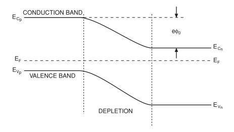
Figure 2.9 Energy band diagram for a P-N junction
