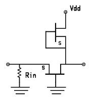
Figure 5.40 IF amplifier matching stage
