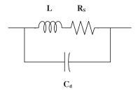
Figure 4.31 Inductor equivalent circuit
