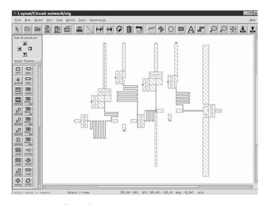
Figure 4.74 Layout representation of a power amplifier
