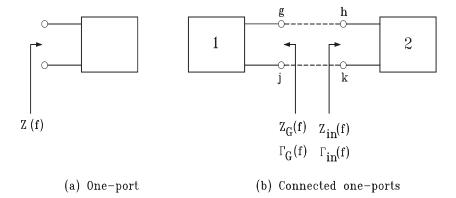
Figure 4.9 Tests for oscillation: definitions of quantities
