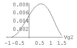
**Figure 5.38** IF output power vs  $V_{g2}$
