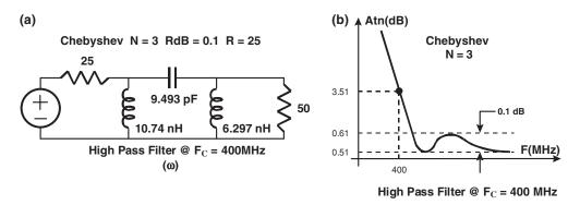
Figure 6.49 Chebyshev filter frequency translation example
