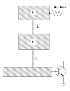
Figure 4.60 LPF using distributed elements
