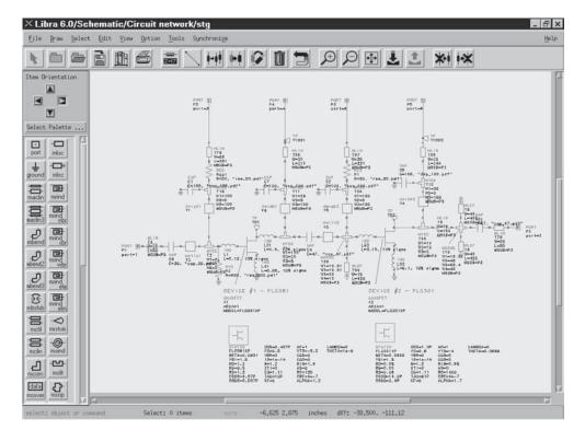
Figure 4.73 Schematic representation of a power amplifier
