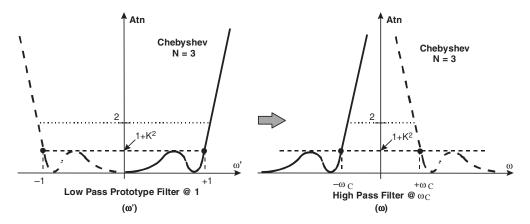
Figure 6.47 LP to HP Chebyshev filter transformation
