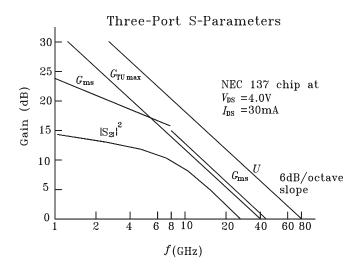
Figure 4.15 Dependence of gain on frequency for typical MESFET
