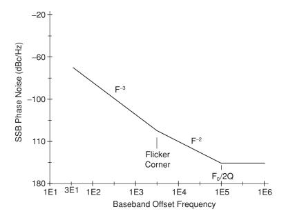
Figure 7.55 Oscillator response with up-converted noise
